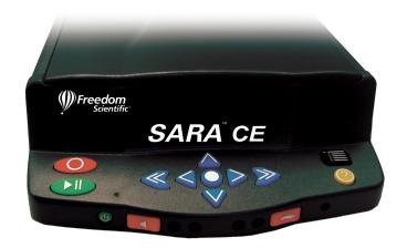
Large color-coded keys with raised markings make operation simple
